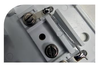
**MECHANICAL:** One or two button operation. When activated, it displaces the magnet from the reed switch or activates the microswitch. Mechanical panic buttons are reset by key repositioning.
